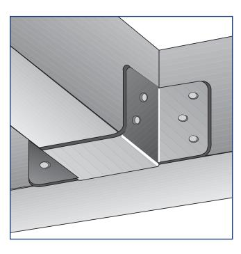
Light duty applications, the speedy minor can accommodate a joist depth of up to 100mm.
