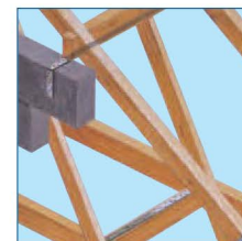
Anchorage of gable end to roof structure.
