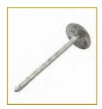
The Spring Head Nail is most commonly used for the application of galvanised sheeting onto timber frame. This nail allows for some structural movement without loosing any strength. Spring head nails have a spring head washer.
