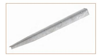
A Sturdy galvanised steel pin, designed to be driven into soil to secure log border roll. Simply insert the pin into the soil and nail or screw through the pre-punched holes into the timber.
