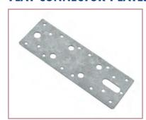
A range of pre-punched flat connectors suitable for many timber to timber, masonry or steel applications. Manufactured from 2.5mm thick galvanised steel as standard.
