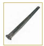
Flooring Brad Nails 65mm - Steel flooring brads are most commonly used to nail floor boards. The L shaped head reduces damage to the floorboards when being fixed in place and also allows for an easy removal of the boards if necessary.
