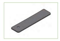
Debonding sleeves are used on plain-ended wall ties at vertical movement joints in a run of brickwork or blockwork. They should be installed with a 10mm gap at the end to allow for expansion of the masonry.
