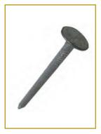
Alternative to copper nails and is used for fixing slates to timber. This multipurpose nail has a galvanised, rust resistant finish.
