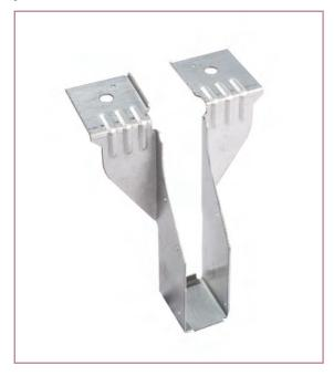
Traditional timber to masonry hanger range for building into brickwork or blockwork. All Hangers require 675 mm (3 courses) of Masonry above. The masonry must be cured for 28 days prior to loading the floor.
