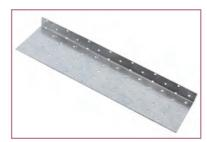
Splice plates are used for the butt jointing of timbers with similar cross section. Normally used to replace rotten or burnt timbers.
